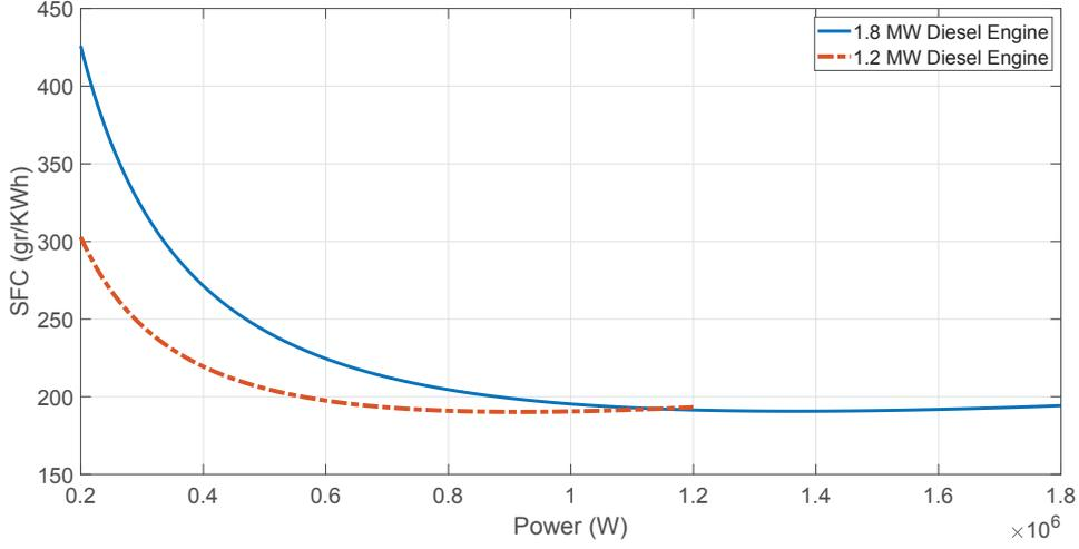
Figure 4.3: SFC curve of two diesel engines with different power ratings [27].
