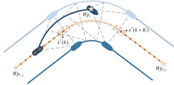
(b) Smooth trajectory with kinematic interpolation.
