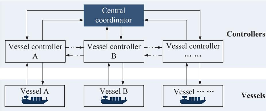
Figure 2.6: Structure of Multi-layer negotiation methods.
