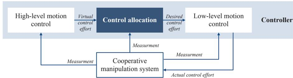
Figure 2.7: Generic control structure of cooperative manipulation.
