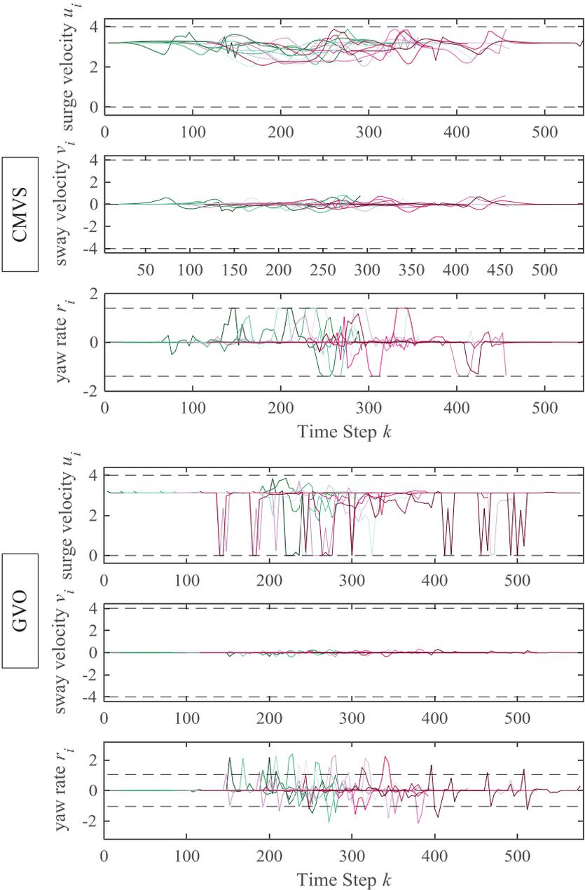
Figure 6.9: Linear and angular velocities of the ASVs that have the same dynamics with CyberShip 2 using the proposed method and the GVO method. For the legend, see Figure 6.6.
