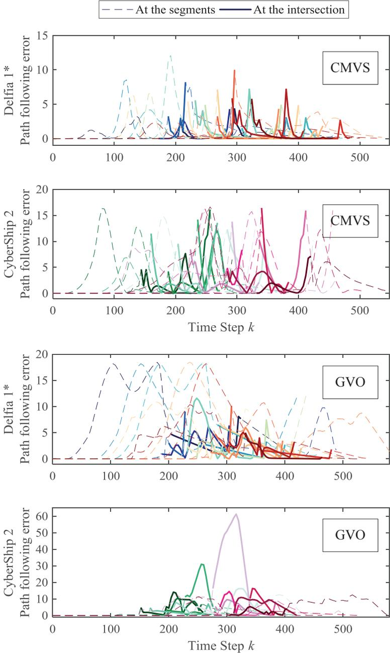
Figure 6.7: Comparison of path following errors of ASVs using CMVS and GVO. For the legend, see Figure 6.6.
