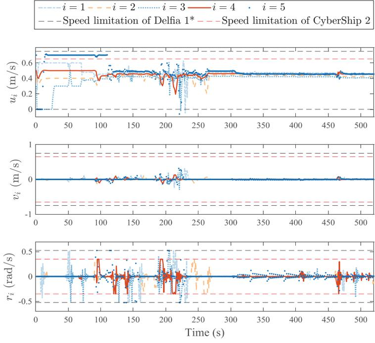
(a) Linear and angular velocities of the ASVs using Speed-based VTF.
