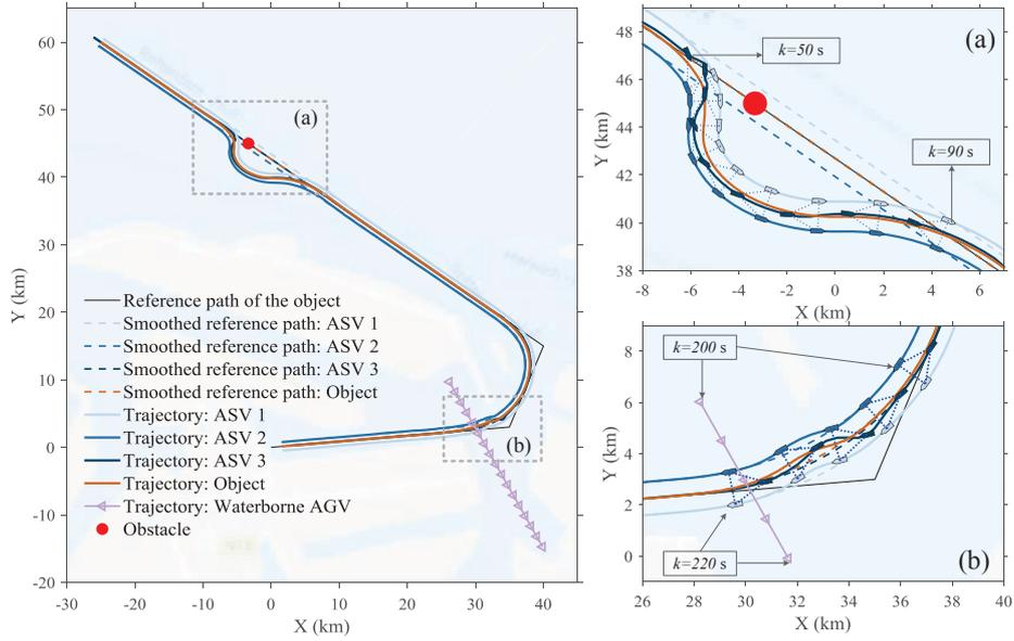
Figure 5.7: Trajectories of the ASVs and the object.
