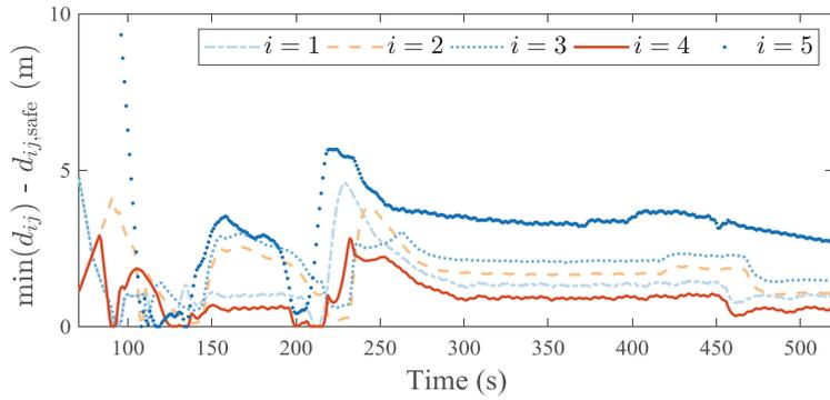
(a) Distance between an ASV and its nearest neighbor using Position-based VTF.
