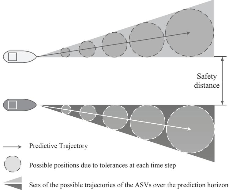
Figure 4.4: Adjustment on safety distance due to feasibility tolerances.
