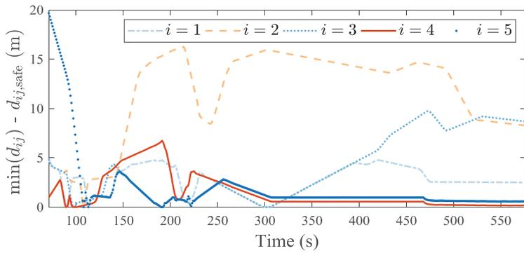
(b) Distance between an ASV and its nearest neighbor using Speed-based VTF.
