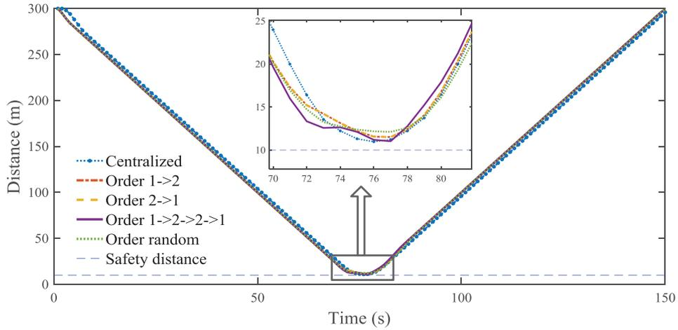
Figure 4.7: Relative distance with different updating sequences.
