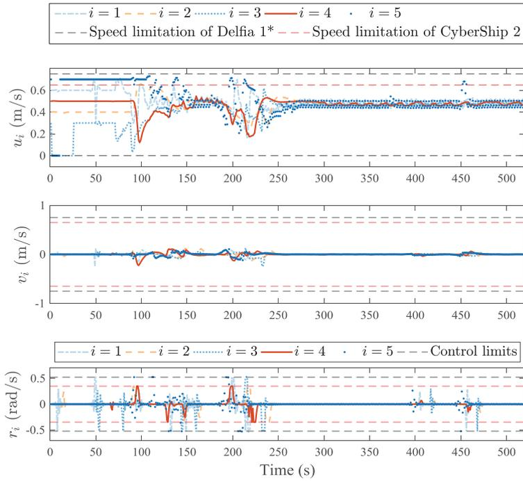
(a) Linear and angular velocities of the ASVs using Position-based VTF.
