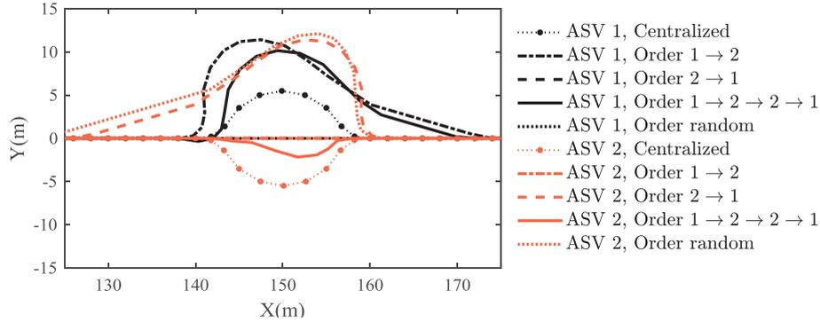
Figure 4.5: Trajectories of each vessel with different updating sequences.
