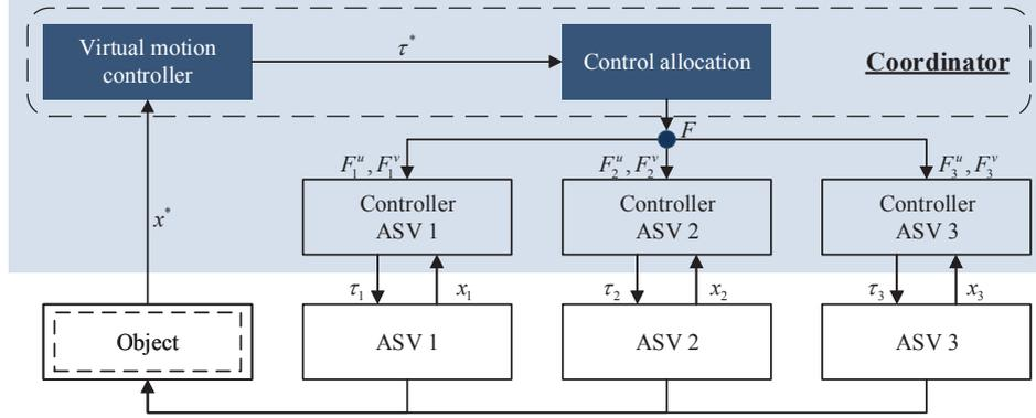
Figure 5.3: Multi-layer DMPC for cooperative object transport.
