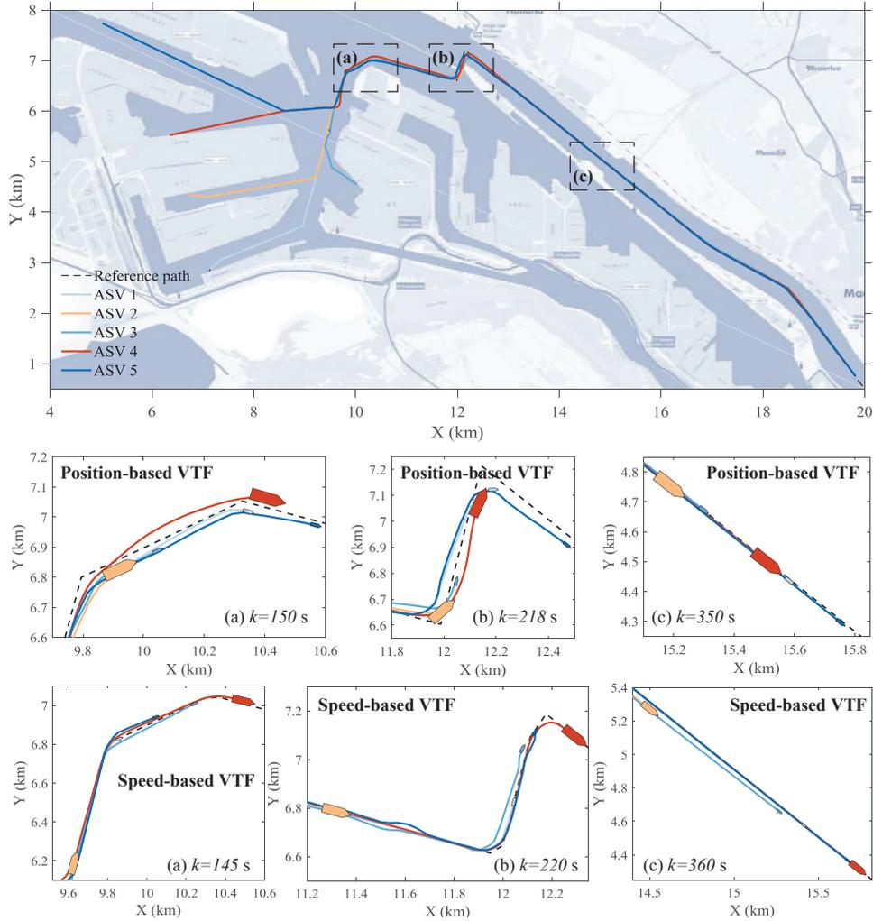
Figure 4.17: Trajectories of the ASVs.
