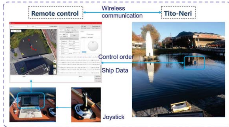
Figure 18: Sailing data collection of Tito-Neri ship in the open pool in Delft University of Technology.
