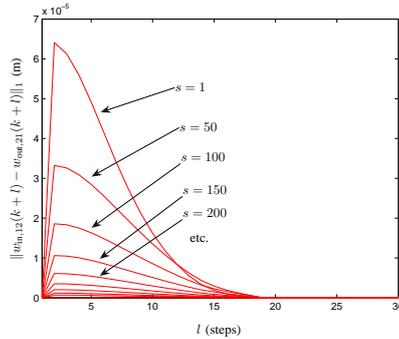
Fig. 5. Evolution at  $t = 2.23$  of the absolute error (1-norm) between the interconnecting output of controller 1 and the interconnecting inputs of controller 2, i.e., the values that both controllers would like to give to the interconnecting variables  $\Delta e_4(k+l)$ , for  $l = 1, \dots, N$  over the iterations.
